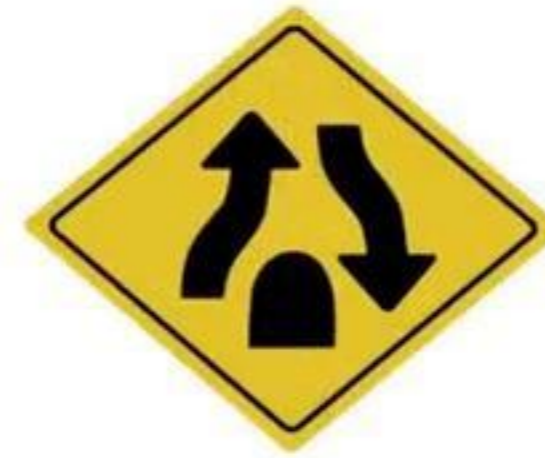
Divided road ends
