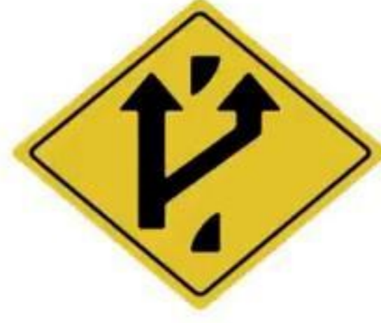
Parallel right exit to the main road
